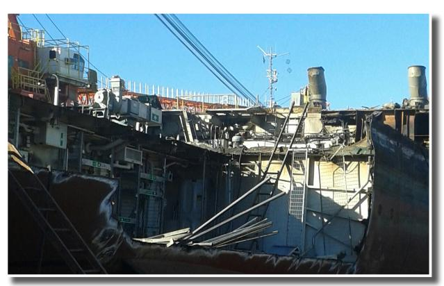
14 Jan 2016 – Ex HMS York showing remains of the engine room. The vessel is dismantled from 'top to bottom' while afloat and from 'bow to stern' on the dry slip way.
