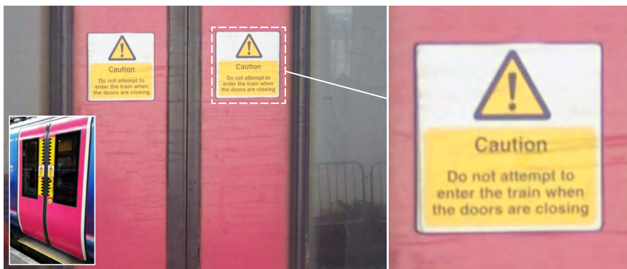
Figure 24: Cautionary sticker on the outside of the class 165 trains requesting passengers to not attempt to board the train when the doors are closing. Inset image showing 'sharks teeth' graphic design on the livery of a TransPennine Express train to warn passengers of the dangers of obstructing a door.
