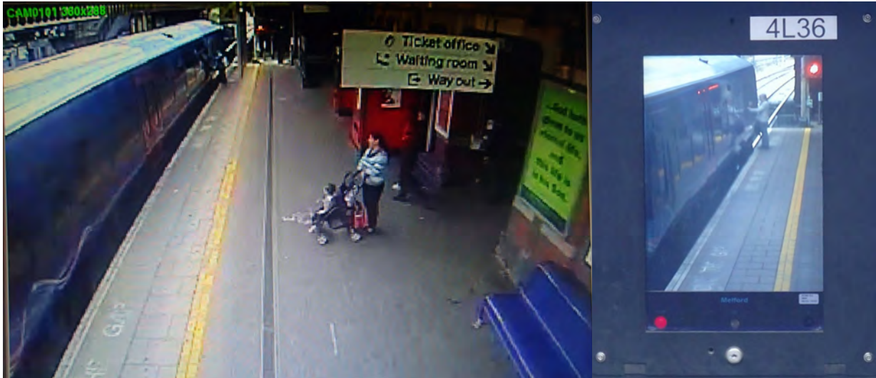
Figure 29: (a) showing the passenger at the rear portion of the train on the platform CCTV image (courtesy of GWR), and (b) an image taken during the RAIB reconstruction of the events at the same location on platform 4 (from the driver's view of monitor 4L36)
