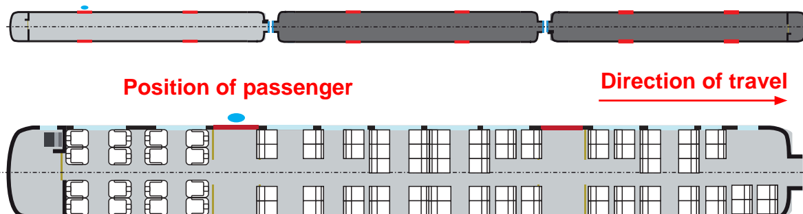
Figure 4: Class 165 vehicle layout and position of passenger attempting to board the rear set of doors of the carriage
