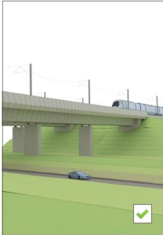
Refinement of abutment design: bank seat abutments, visible extent of concrete abutment minimised., © Grimshaw
