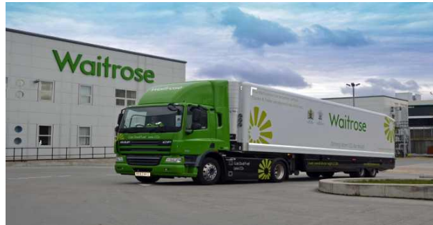
Dual fuel diesel/gas truck and low carbon trailer combination operated by Waitrose
