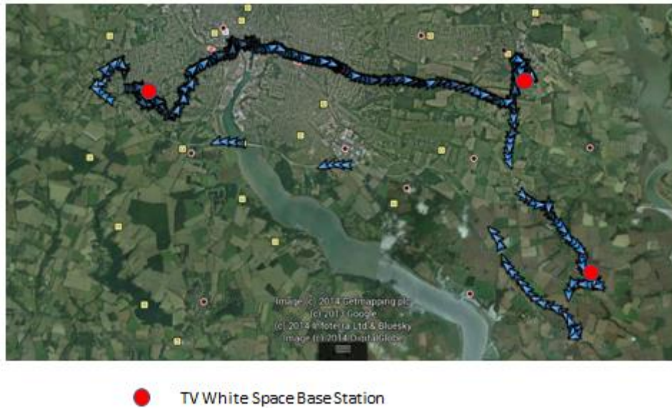
Figure 15: Coverage obtained from TVWS base station on roads around Ipswich
