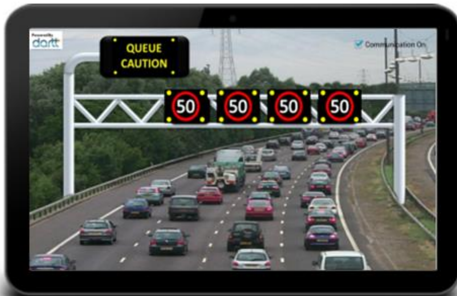
Figure 8: Example Gantry signs displayed
