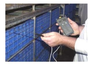
Diagram 6: A portable temperature and humidity sensor being used in the birage
