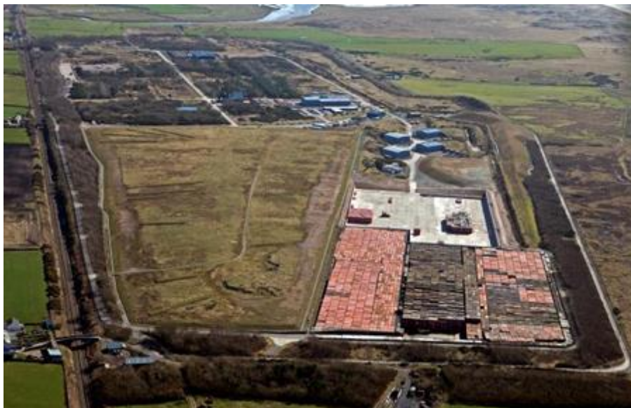
Figure 4-4 LLWR Site. Previous trench disposals are located under the grassed area on the left; Vault 8 is almost full and shown bottom right; Vault 9 is indicated by the concrete pad (Courtesy LLW Repository Ltd)
