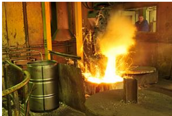
Figure 4-3 Metal melting at the Siempelkamp facility, Germany (Courtesy Siemplekamp)
