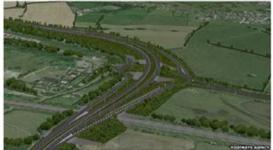
Plans at Little Eaton would see the A38 taken above the A61 to separate local and through traffic
