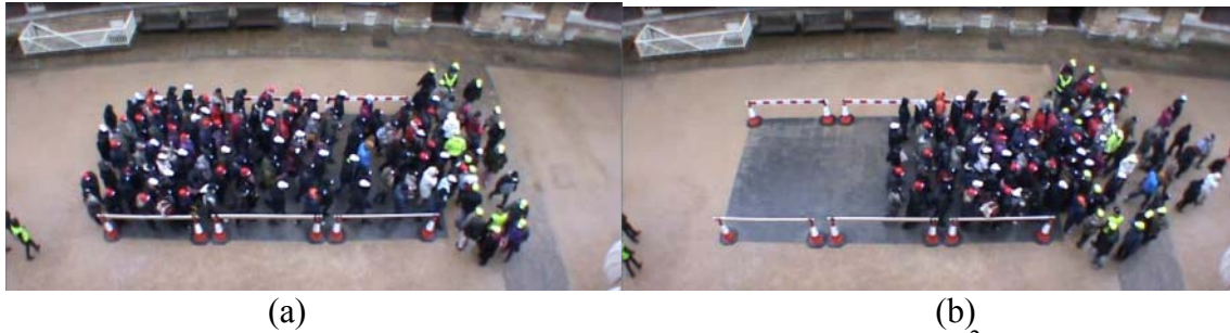
Figure 109: Congestion produced during cross walk trials with 4p/m^2 as (a) population initiates movement, (b) congestion builds at cross-walker position.
