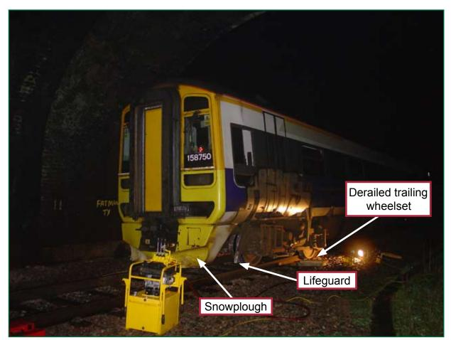
Figure 3: Leading end of Unit 158750 and derailed leading bogie
