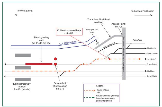
Figure 2: Track diagram of the area in which the accident occurred
