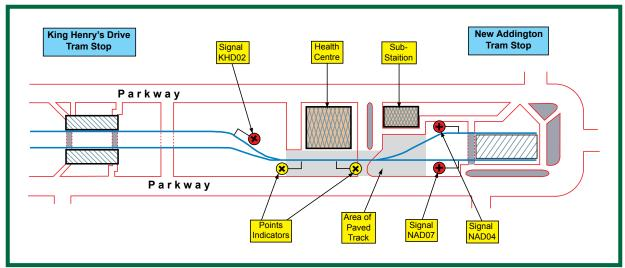
Figure 4: Diagramatic representation of the line between King Henry's Drive and New Addington
