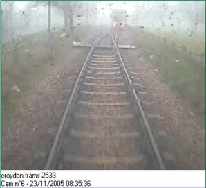
Figure 9: CCTV record from tram 2533. Tram 2538 clearly foul of running line
