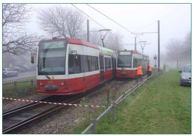
Figure 2: Site of the collision looking towards King Henry's Drive transtop, showing the rear of tram 2533 (on left) and the front of tram 2538 (on right). The rear of KHD02 signal is on the shorter post to the right of tram 2538.
