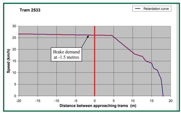
Figure 17: Speed - Distance record for tram 2533 (negative distances are on approach to point of collision)
