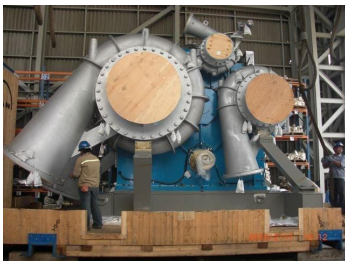
Figure 2.5: Main Air Compressor
