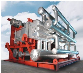
Figure 2.6: Main Heat Exchanger
