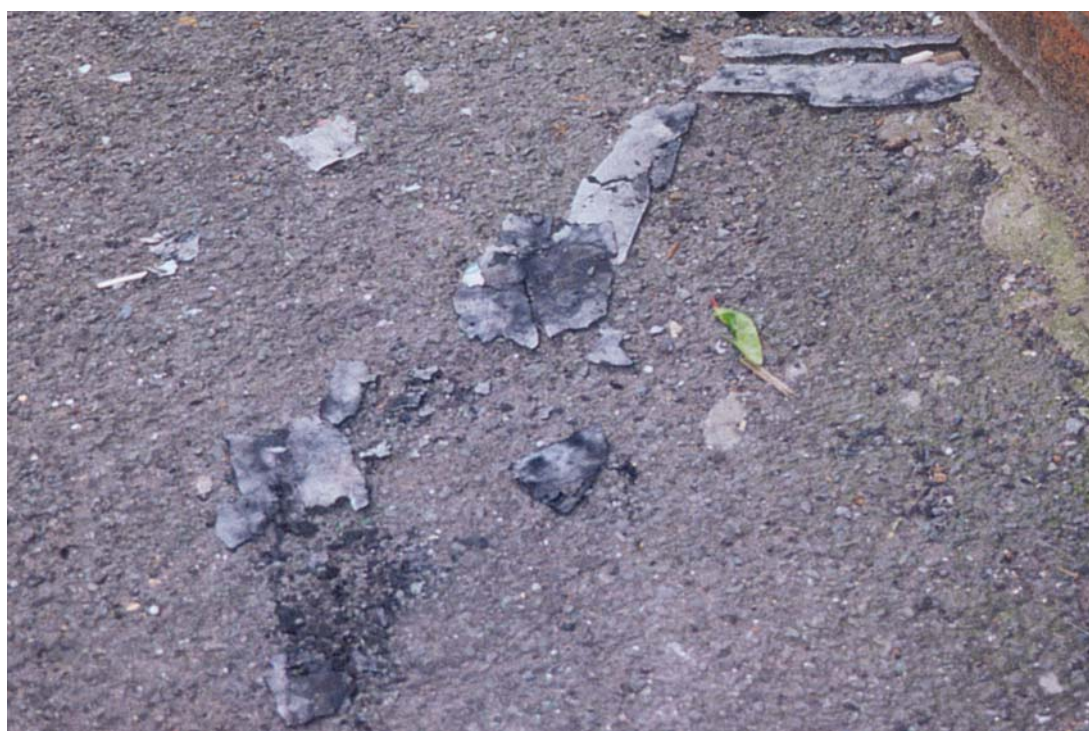
Figure 1 Asbestos containing fallout from large scale industrial fire (Bridgman, 1994) (Published with the permission of S Bridgman and Wirral MBC)
