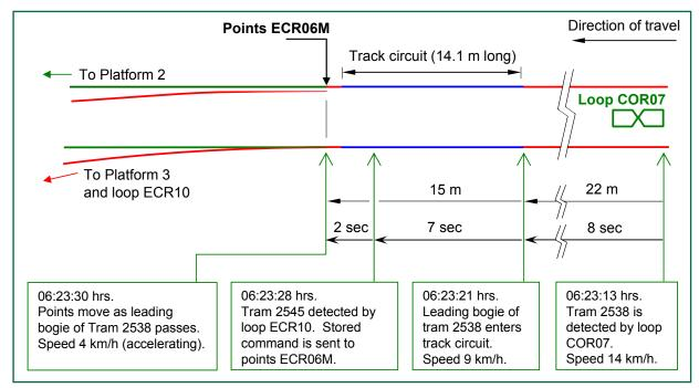
Figure 11: Diagram showing calculated position of tram 2538
