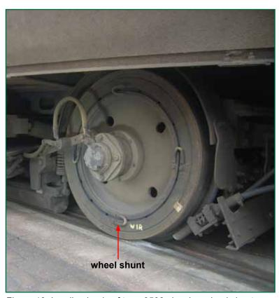
Figure 13: Leading bogie of tram 2538 showing wheel shunt
