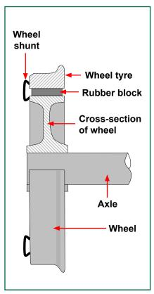
Figure 14: Part-section of wheel
