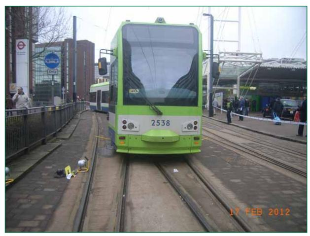
Figure 7: Rear view of tram 2538 following derailment
