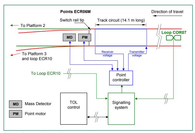
Figure 9: Schematic diagram of the point control system
