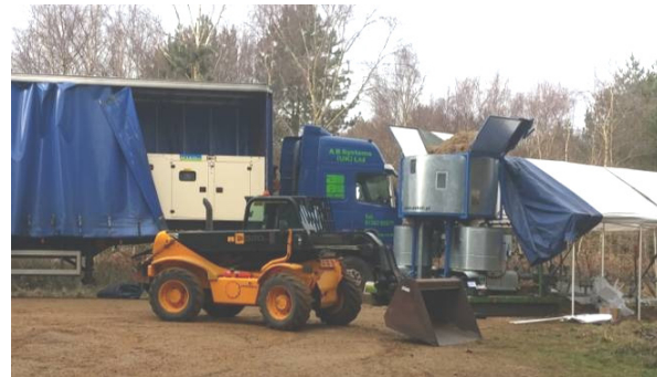
Fig 44 – Telehandler loading arisings into briquetter drum
