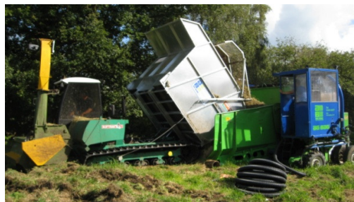
Fig 38 – Softrak depositing directly into feed-table of AgBagging machine
