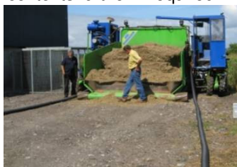
Fig 39– Feeding air pipes through the AgBag
