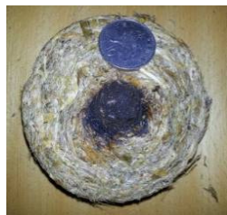
Fig 91 – Briquette becomes too hot in centre
