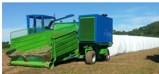
Fig 3– An AgBag machine storing grass silage in AgBags
