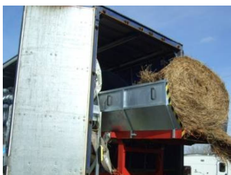
Fig 30 – the shredder at the rear of the original briquetter
