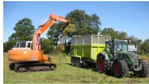
Fig 37– Swing-shovel loading arisings into tractor trailer
