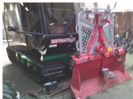
Fig 101– The winch attached to the Softrak
