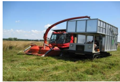
Fig 35– Tracked Dumper collecting arisings cut by PistenBully
