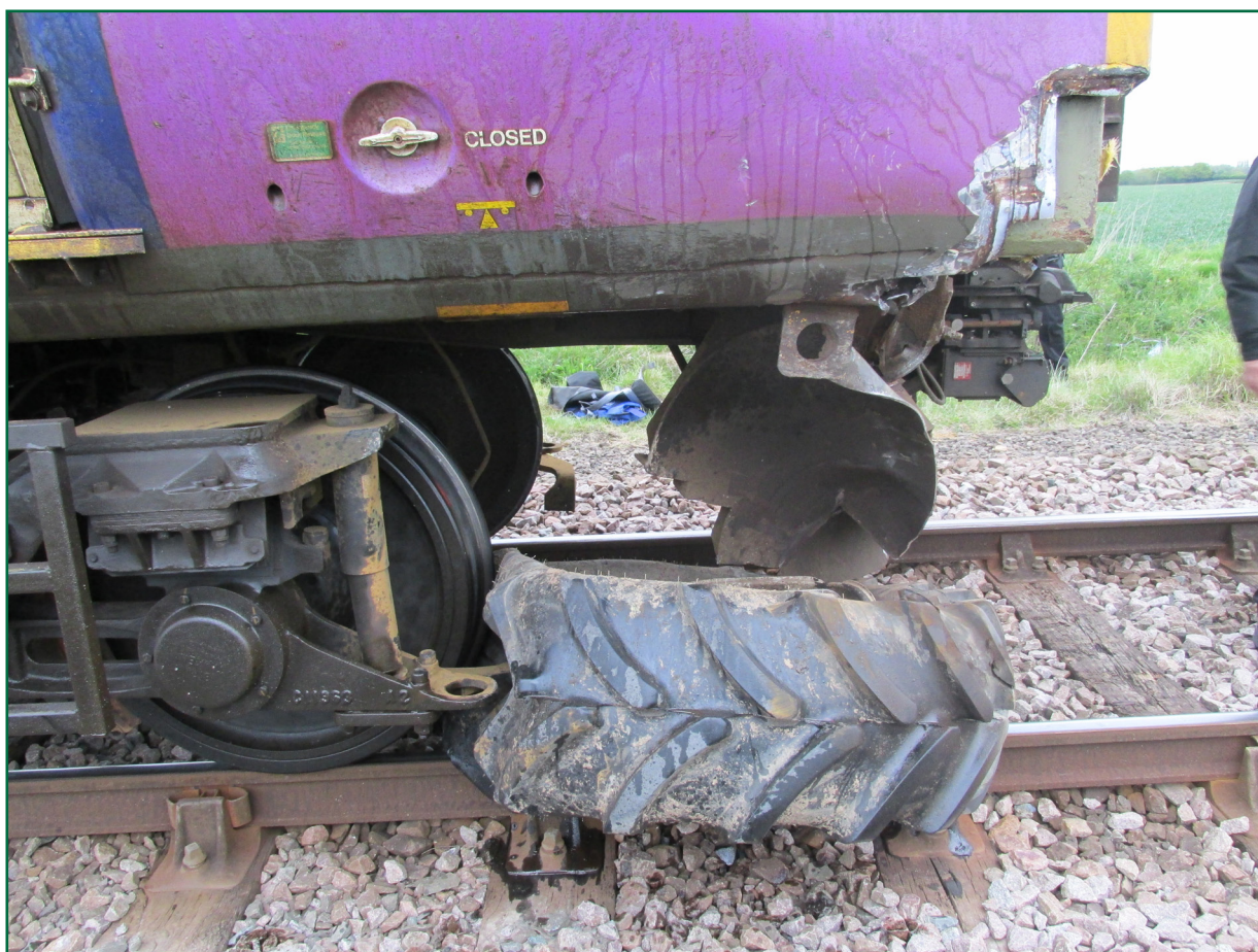
Figure 6: The tractor's front wheel and tyre wedged under the front right-hand side of the train (image courtesy of British Transport Police)
