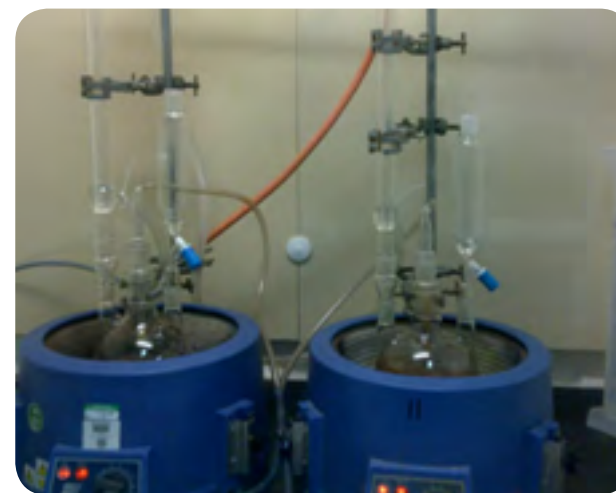
Figure 3 Determination of sulphites as sulphur dioxide by the Monier-Williams method
