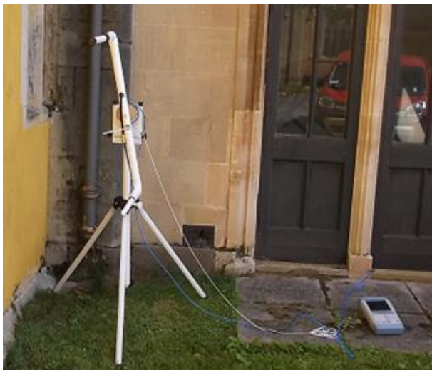
Figure 3 Spectrum Analyser Connected to the Horizontally Positioned Antenna
