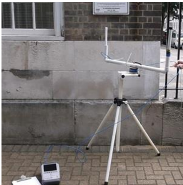
Figure 4 Spectrum Analyser Connected to the Vertically Positioned Antenna
