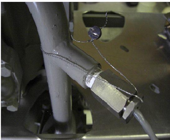
Figure 62 Typical installation of temperature sensor and sealing arrangement
