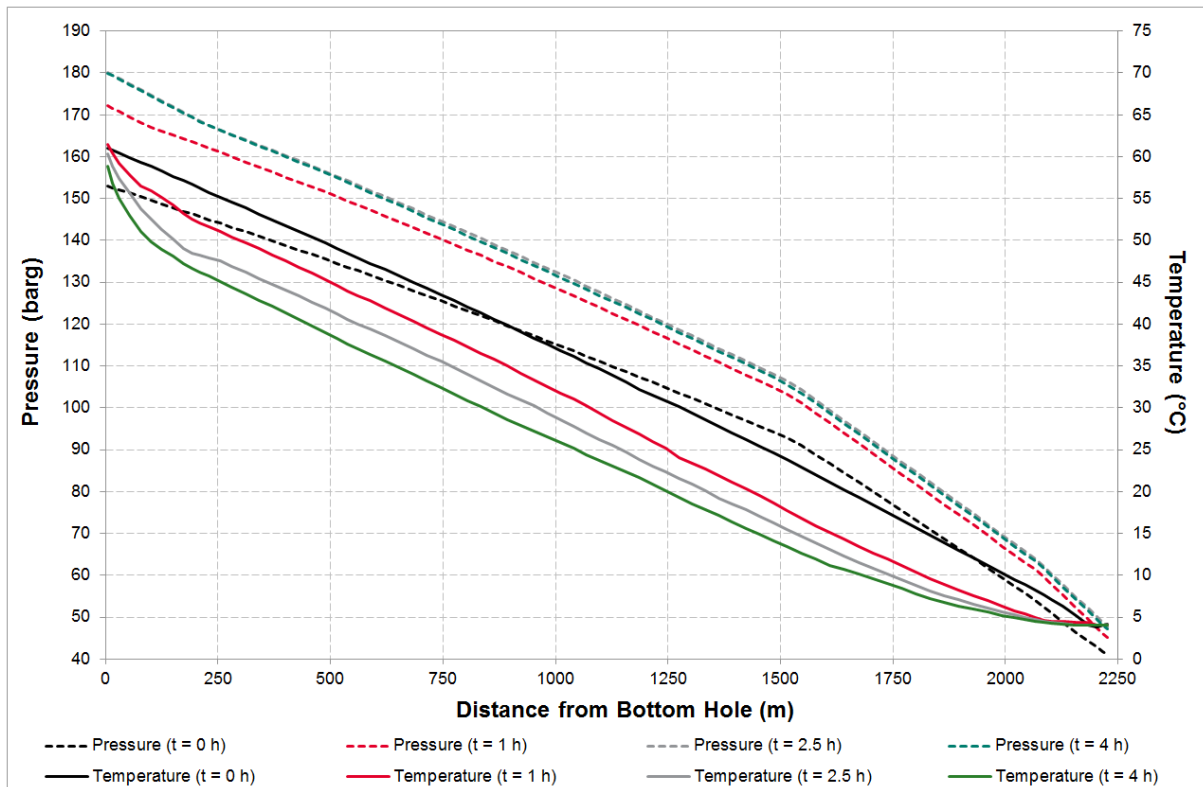
Figure 7.70: Pressure and Temperature Profiles during Prewash MEG Flush with an Injectivity of 7.7 \times 10^{-7} kg/s/Pa, 150 barg Reservoir Pressure, Winter Conditions
