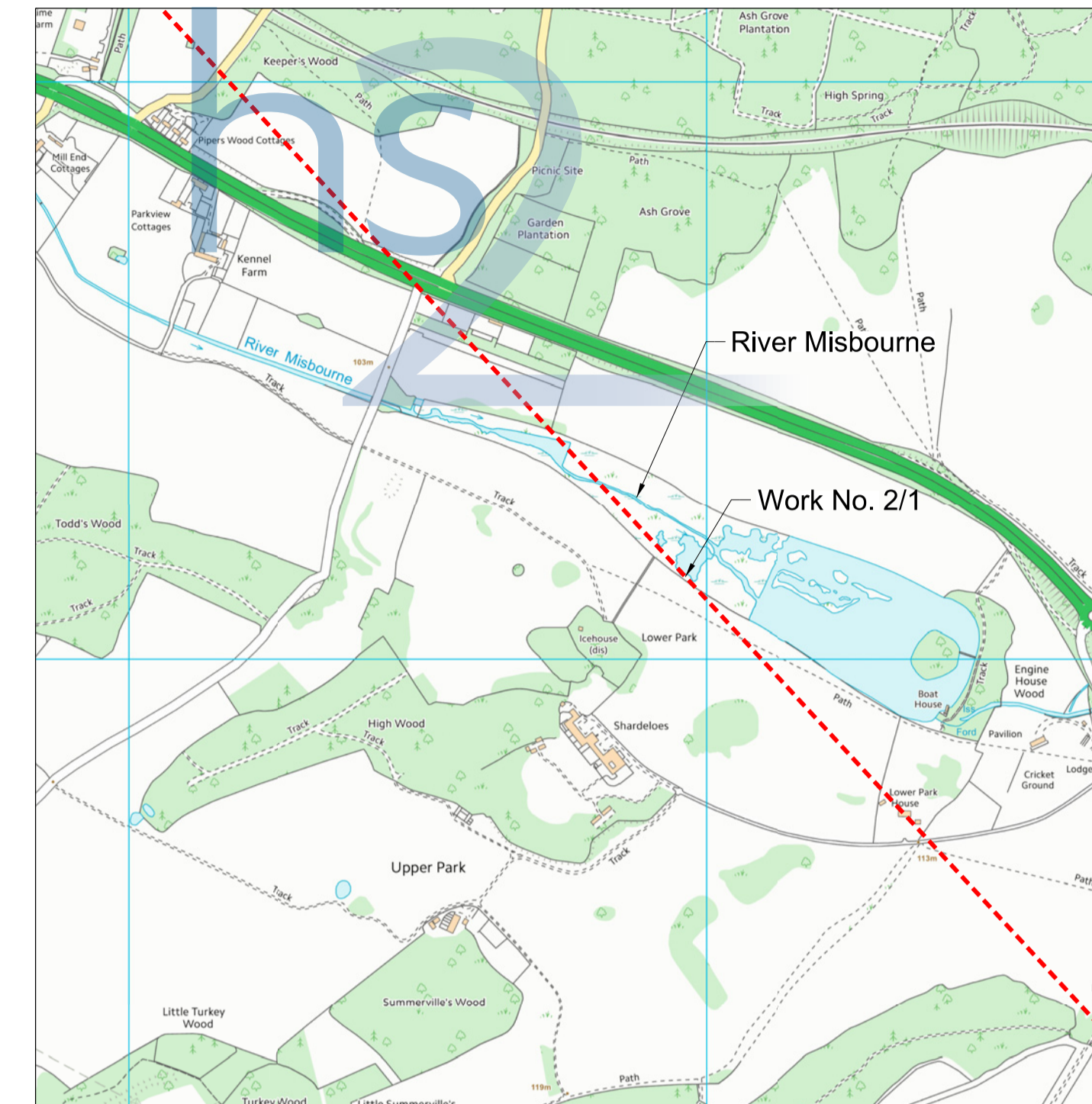
Proposed Tunnel under River Misbourne
