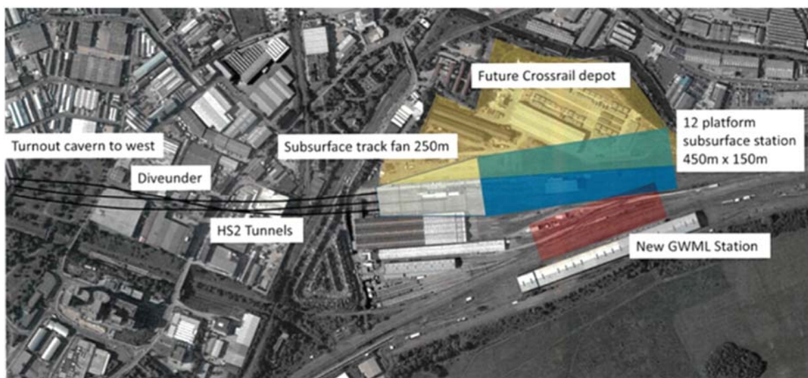
Figure 4 Indicative footprint of a 12-platform station at Old Oak Common
