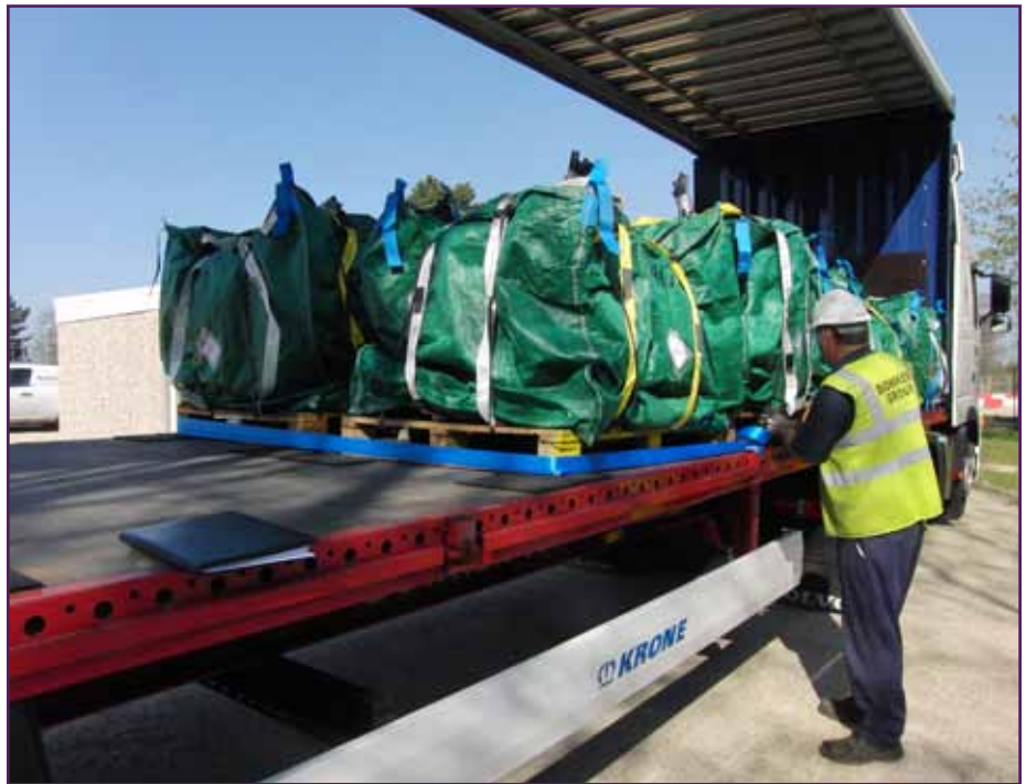
Soft-sided waste bags are loaded onto a transport vehicle
