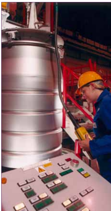
Above: Waste can be encapsulated in 500-litre drums.
