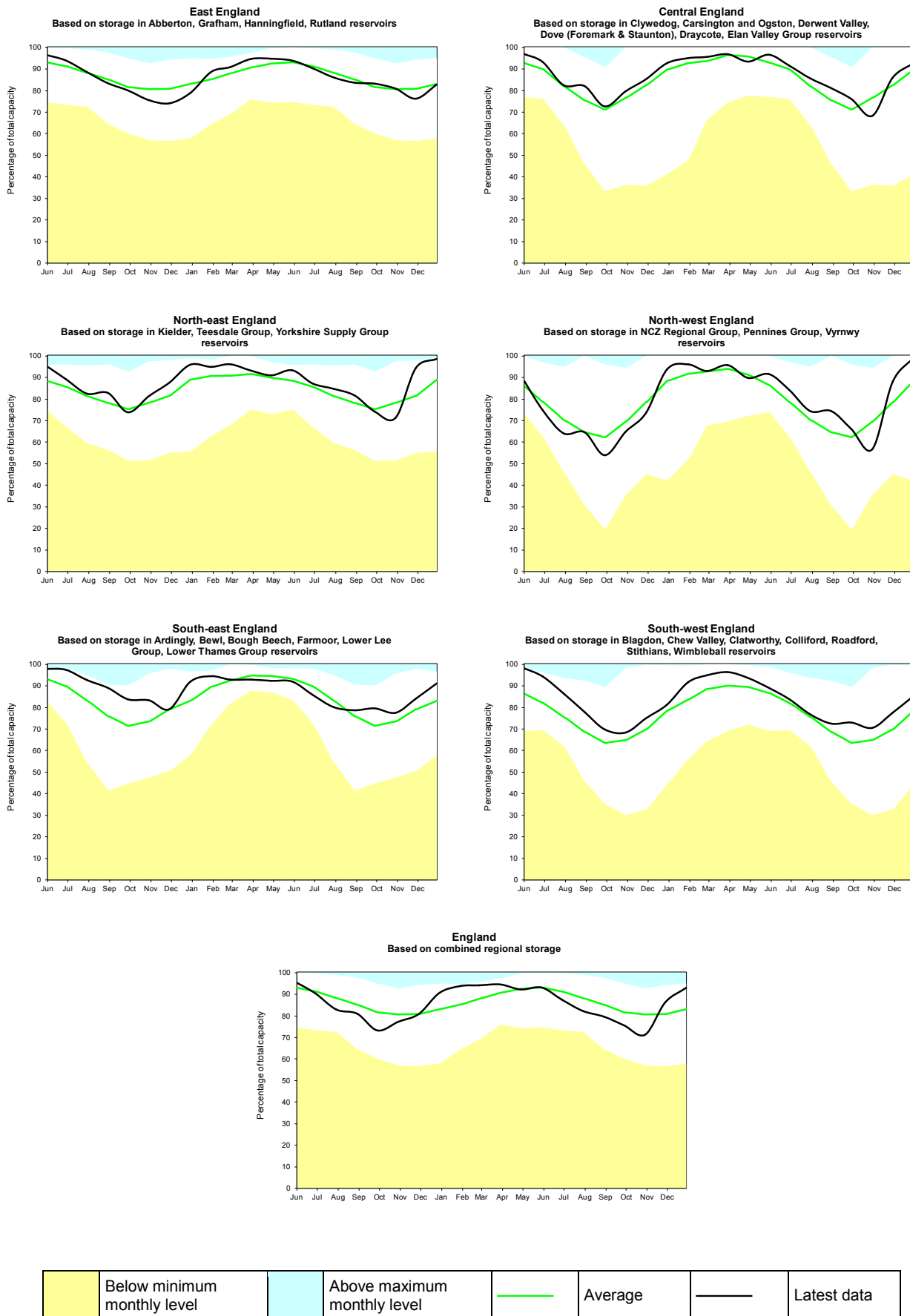
Figure 5.2: Regional reservoir stocks. End of month reservoir stocks compared to long term maximum, minimum and average stocks (Source: Water Companies). Note: Historic records of individual reservoirs/reservoir groups making up the regional values vary in length.
