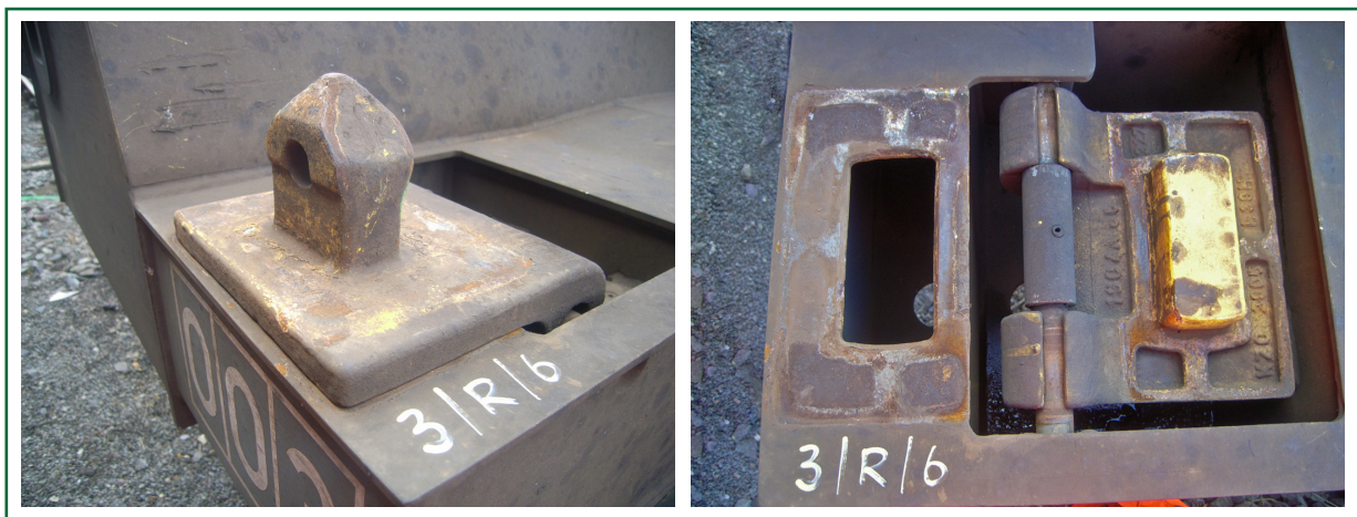
Figure 4: Fold-down spigot with inboard hinge, as fitted to FEA-B and FEA-S wagons, deployed (left), stowed (right)
