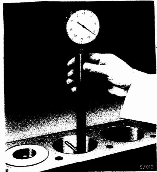
Fig 60 - Checking piston bores
