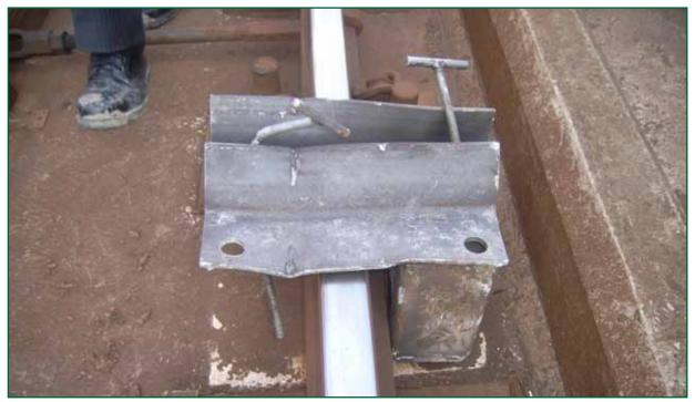
Figure 4: Drilling jig (damaged as a result of the derailment) shown in its operating position with two drilling guide holes showing on the front edge
