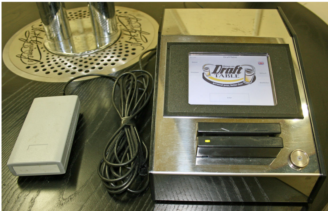
Figure 6 - Remote FR controller box with transceiver.
