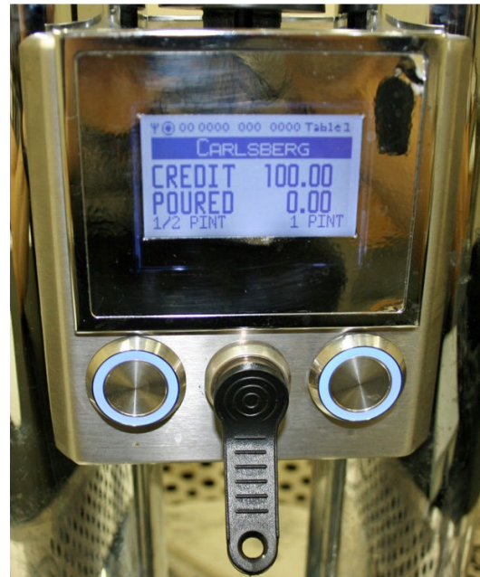
Figure 5 - Central column LCD, magnetic i-Button holder and touch sensitive activation buttons
