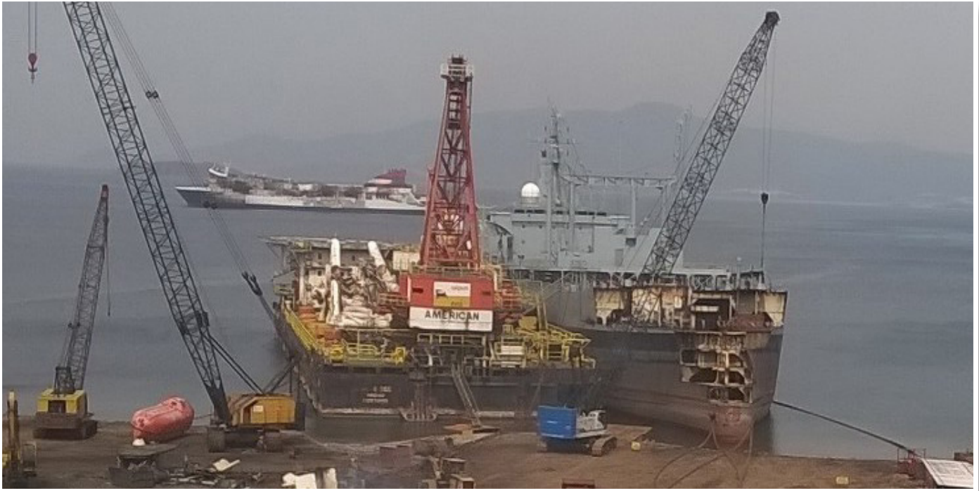
22 March 2016 The first stages of Ex-RFA Orangeleaf being dismantled showing the dismantling of the accomodation and bridge.
