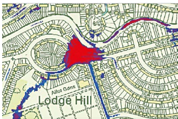
Figure 4 - In 2014 we built a comprehensive digital model with Birmingham City Council to understand the causes of the flooding which occurs in the Lodge Hill area of Birmingham during heavy rainfall events. Working together to understand the various causes of flooding and evaluate the solutions makes it more likely we can identify and address the root causes of flooding.
