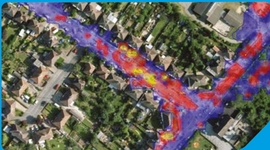
Flood risk mapping in Holt Drive, Leicester. Areas in red at risk of internal flooding. Model used to inform investment.
