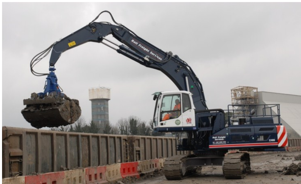
Figure 3.18 Grab handling of material from rail wagons
