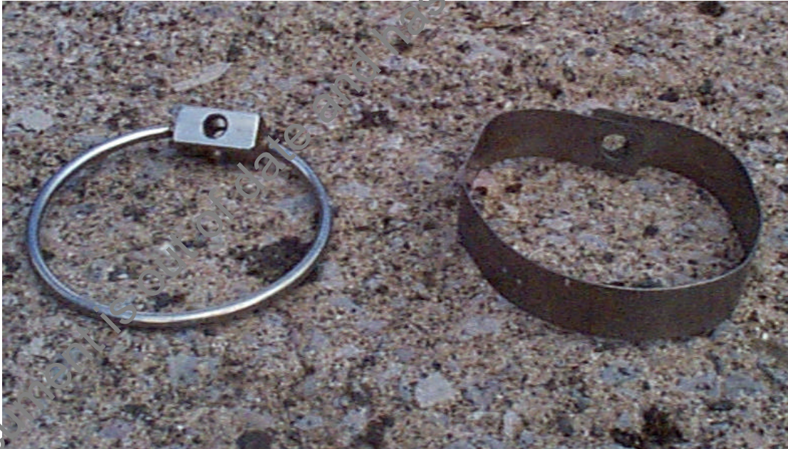
Figure A3.2 Close-up of small diameter (100 mm) anodes tested. These small diameter anodes are used specifically for fry sampling where high voltage gradients are required.
