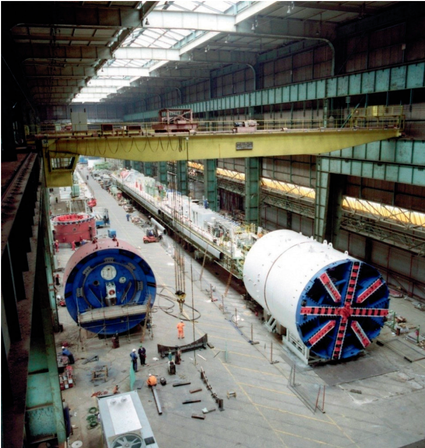
Figure 21: Photograph of a typical tunnel boring machine
