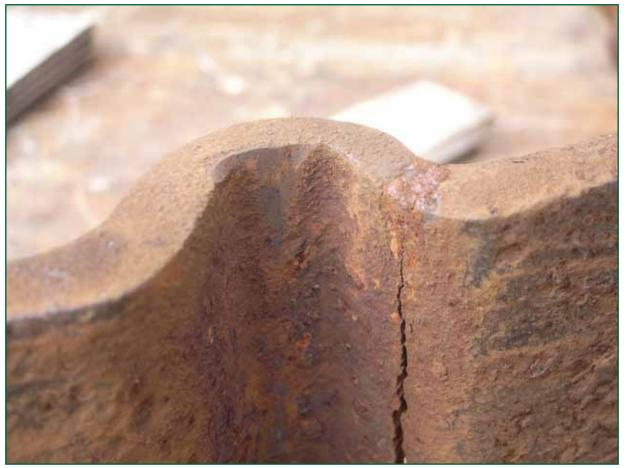
Figure 5: Failed baseplate after removal from the track
