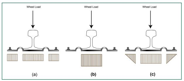
Figure 6: Pressure distributions beneath baseplate
