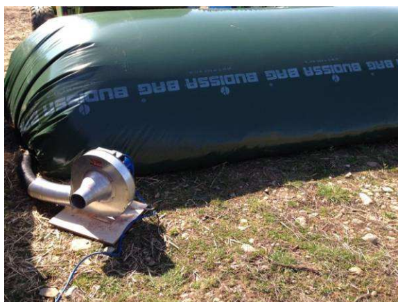
Figure 41a 1.5kW fan used to circulate air
