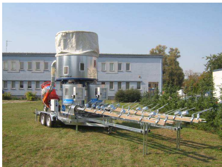
Figure 43: Mobile briquetter with a throughput of 3,000kg per day
