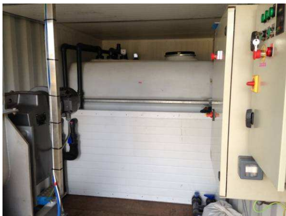
Figure 9: Screw press module housing press fluid storage tanks and screw press
