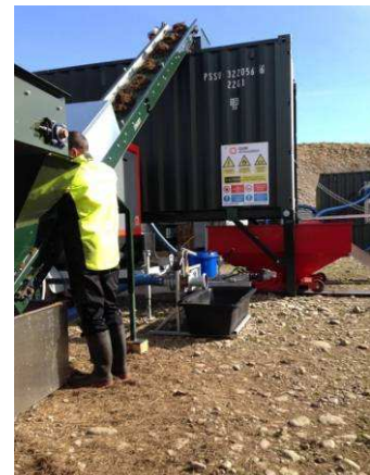
Figure 8: Biomass pre treatment facility with water recycling system and container housing screw press
