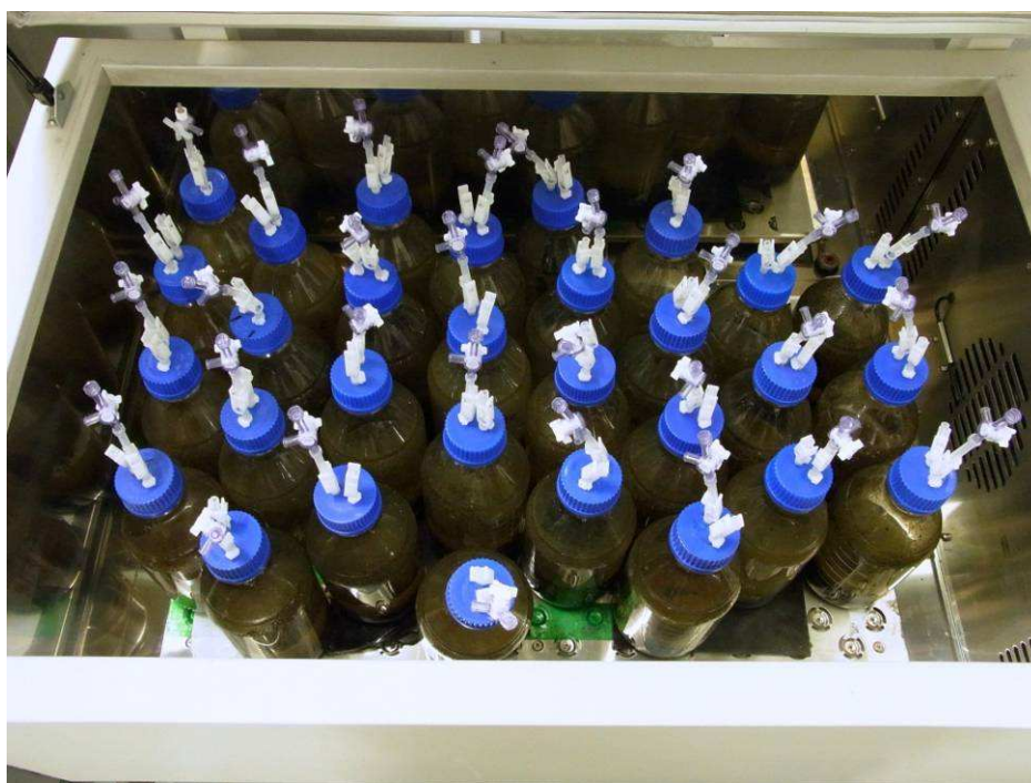
Figure 19: Large lab scale digestions took place in a Brunswick Innova 4300 Incubator shaker.
