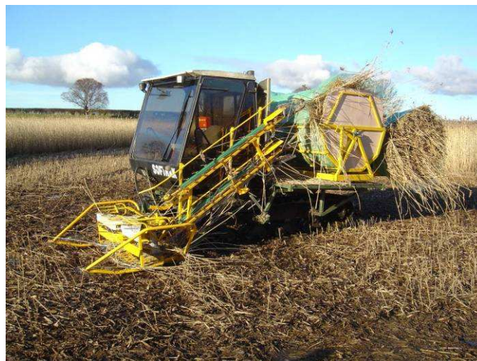
Figure 27: Prototype reed cutter binder developed by Loglogic with AMW's baler and rear extension platform
