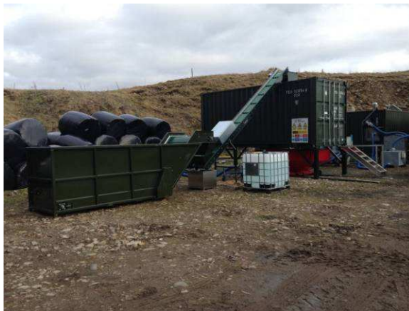
Figure 8: Biomass pre treatment facility with water recycling system and container housing screw press
