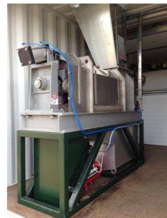
Figure 9: Screw press module housing press fluid storage tanks and screw press
