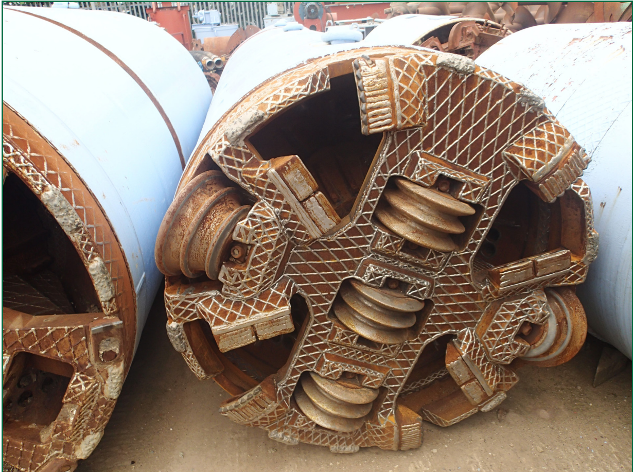
Figure 10: TBM cutter head
