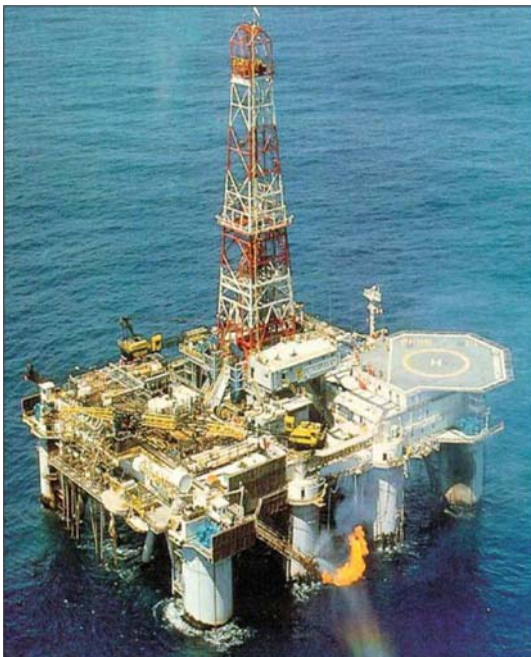
Figure 4: Example of semisubmersible platform.
