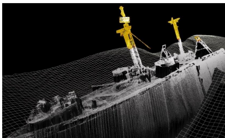
Fig. 21 Laser and multibeam data of the forward section
