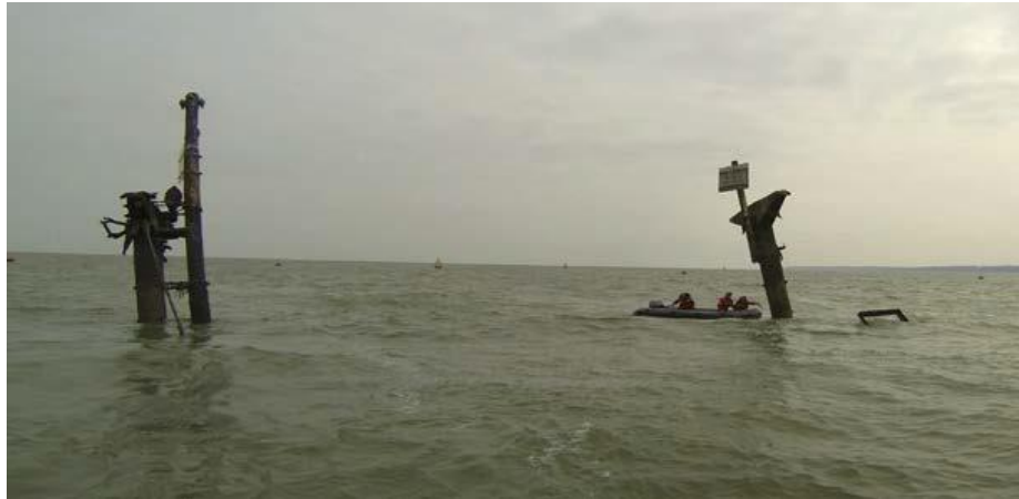
Fig. 35 Taking surface mast thickness readings
