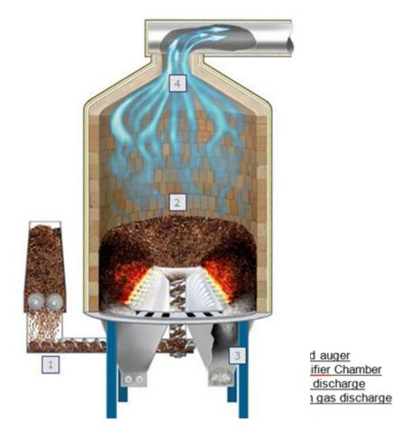
Ignition of the wood (by natural gas) occurs once required temperatures (850°C) are met within the secondary combustion chamber by pre-heating with natural gas. Where required, heat can also be supplied within the transfer
