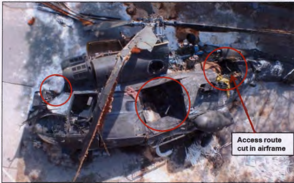
Figure 1.4.40 - Extraction routes for XW229's occupants
