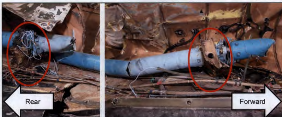
Figure 1.4.34 - TRDS Bearings and flexible coupling damage
