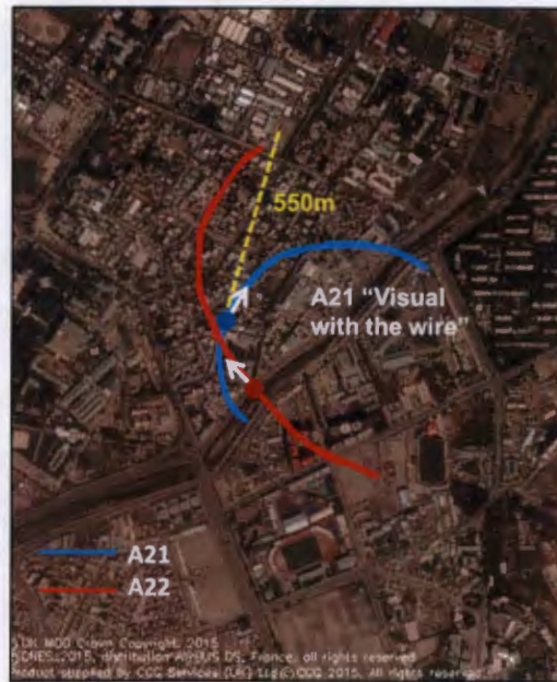
Figure 1.4.20 - Relative positions of aircraft and tether when A21's Captain stated that he was visual with the wire
