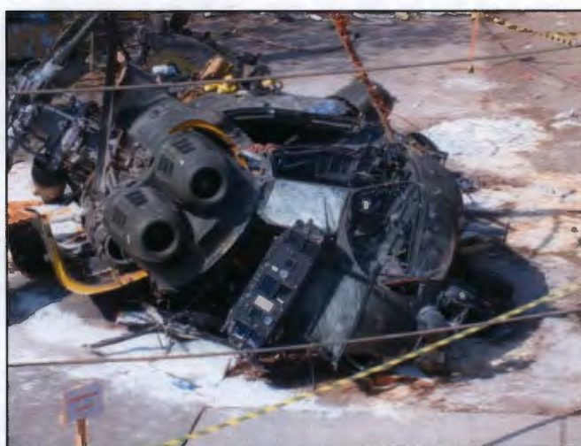
Figure 1.4.38 - Distortion to XW229's airframe
