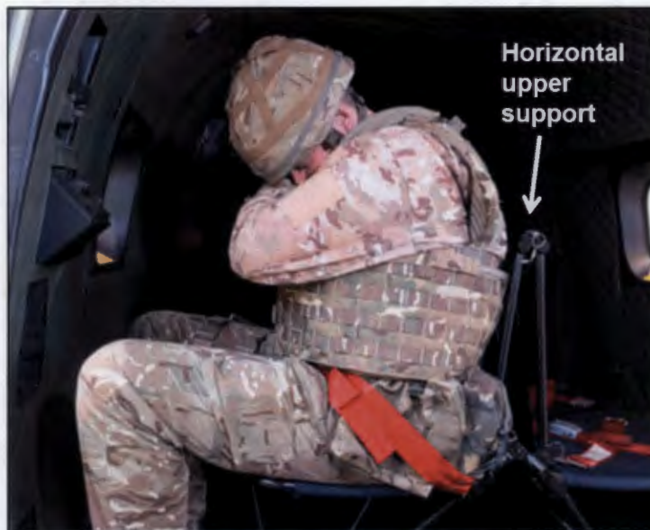
Figure 1.4.50 - Position of troop seat upper support
