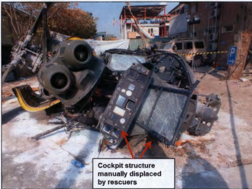
Figure 1.4.41 - Displacement of cockpit structure
