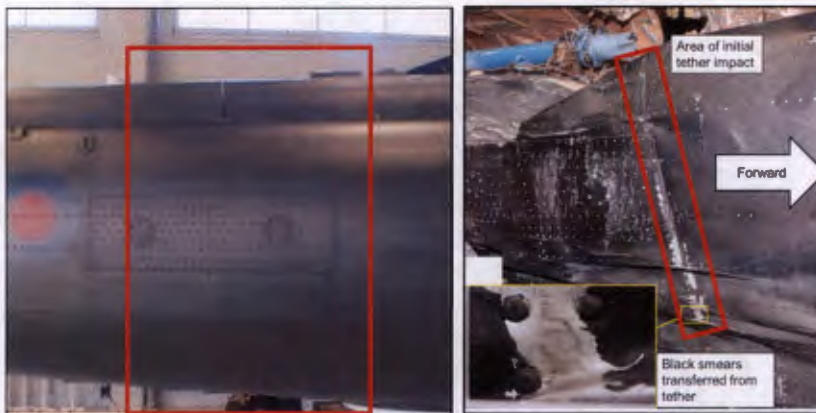
Figure 1.4.23 - Images showing right side of an undamaged tail cone and post tether impact damage to XW229
