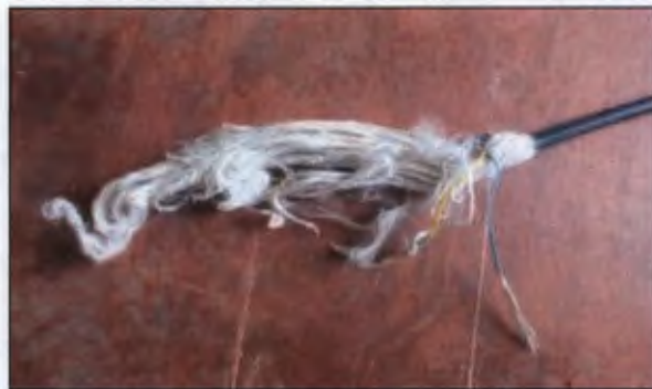
Figure 1.4.22 - PTDS tether at point of failure
