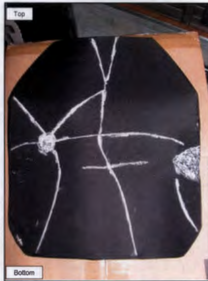
Figure 1.4.49 - Fracture Damage to Passenger C's rear ballistic protection
