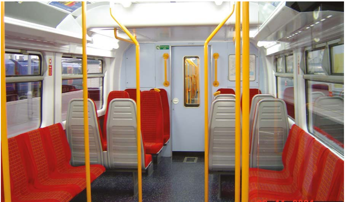
Fig 4.1 Example of an alternative seating layout which allows more comfortable standing room on some shorter distance services
