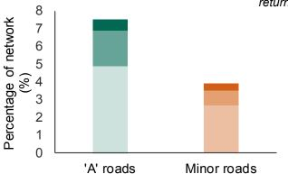
The most common treatment used on both road types in 2014/15 was surface dressing (layers of chippings and binder), followed by resurfacing, then strengthening (reconstruction and overlay). Surface dressing accounted for 65 per cent and 69 per cent of all treatment on the principal 'A' road network and minor road network respectively.
