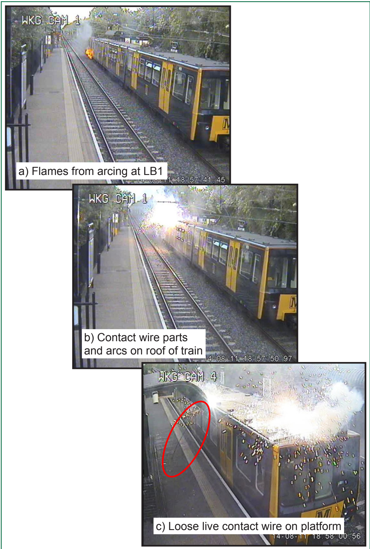
Figure 8: Sequence of events during accident (images courtesy of DB Regio Tyne & Wear Ltd)
