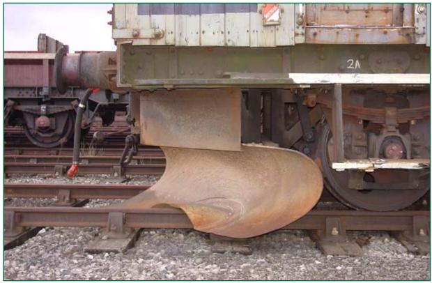
Figure 3: Detailed view of the ballast plough
