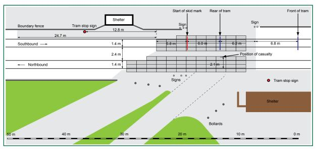
Figure 7: Layout of Norbreck tram-stop and crossing
