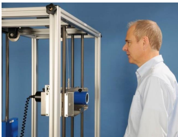
Figure 3: Set-up for measurement of gamma emitting radionuclides in the whole body
