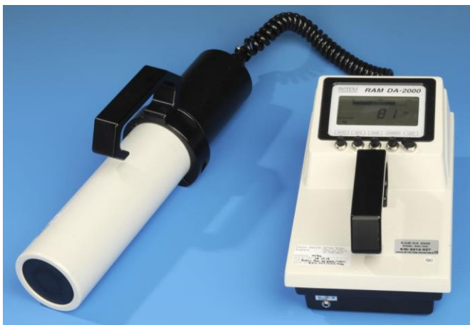
Figure 2: PM11 scintillation probe and DA-2000 survey meter
