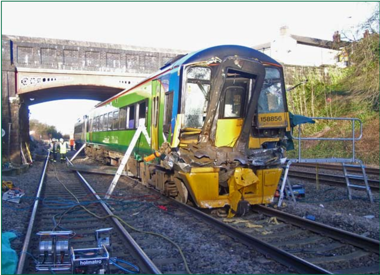
Figure 2: View of the train following collision with the footbridge
