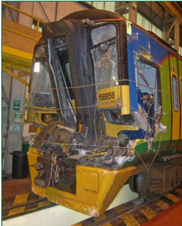
Figure 5: Damage to the leading end of vehicle 1
