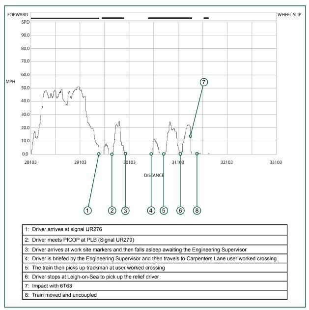
Figure 5: OTDR diagram from train 6T64 showing train speeds and locations within the Leigh-on-Sea possession and work site
