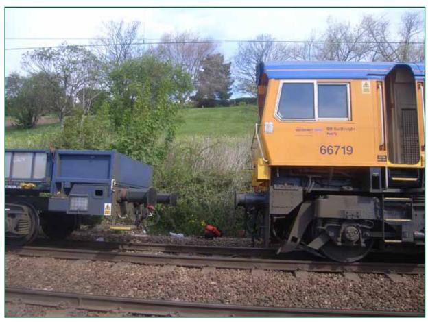
Figure 7: Rear cab of front locomotive of 6T64 after collision
