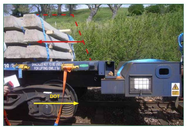
Figure 8: Rear wagon of 6T63 showing the direction of travel (yellow arrow) and the movement of the load (sleepers) from its original position to its final position after the collision (red dotted line)
