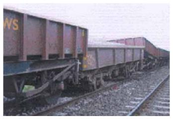
Figure 12: Image of derailed rear wagons of train 6P26 caused by the collision
