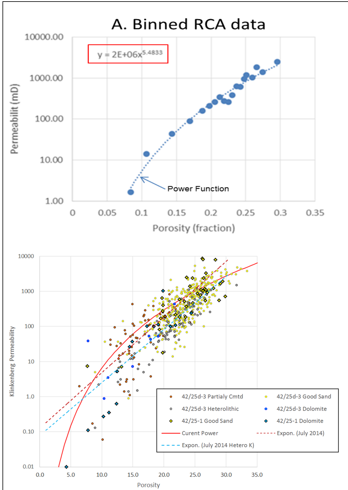
Figure 3.52: RCA (Routine Core Analysis) permeability vs porosity trend function
